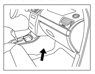
The instrument panel fuse block is located on the passenger's side of the vehicle, on the lower portion of the instrument panel near the floor.
